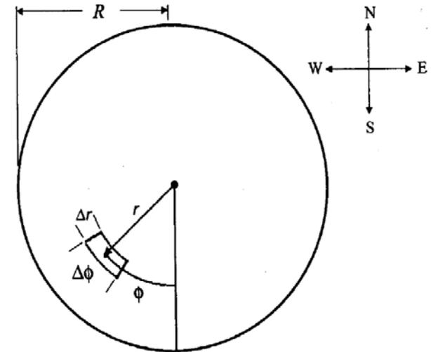
**Schematic of the Tree Trunk Temperature model. Arrows represent direction of heat flow between sections in a tree trunk cross section. The same flows apply for each segment. For the initial model, air temperature is assumed to equal bark temperature and is uniform around the tree trunk.**
